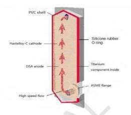
Anode in the electrolyzer is unipolar type. The electrolyzer is upright placed, and the seawater flow through bottom - up one time with a high speed. The hydrogen generated during electrolysis process will outflow with the water flow, and will not store up in the electrolyzer. The high speed water flow will retard the depositing of the calcium and magnesium sediment and extend the acid cleaning period.
