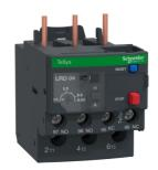
Thermal overload relay, TeSys Deca, 690VAC, 0.4 to 0.63A, 1NO+1NC, class 10A, for unbalanced loads
