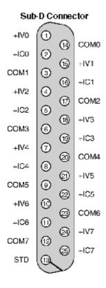
+IVx + Pole voltage input of channel x
