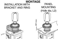
Adaptation for Modulair 107 and 112 ranges To mount the bracket and ring, remove the pressure control knob from the regulator or filter/regulator.
