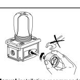
Make sure other unused ports are sealed off on installation
