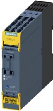
SIRIUS safety relay basic unit 3SK2 series 10 F-DI, 2 F-DQ, 1 DQ, 24 V DC Can be parameterized via SIRIUS Safety ES 22.5 mm overall width screw terminal up to SIL 3 (IEC 62061) up to performance level e (ISO 13849-1) output expansions 3SK1, coupling relay 3RQ1 and fail-safe motor starters 3RM1 via device connector connectable
