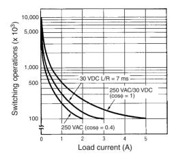
Reference: A maximum current of 0.15 A can be switched at 125 VDC  $(\cos \phi = 1)$  and a maximum current of 0.1 A can be switched if L/R is 7 ms. In
