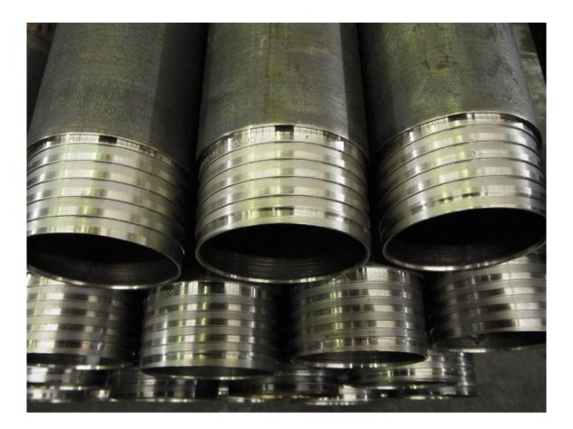
Wireline Drill Rods when used in conjunction with W/L Core Barrels allow the core to be retrieved through the Rods without removing the core barrel from the hole.
