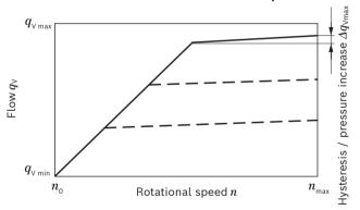
Characteristic curves valid at  $n_1$  = 1500 rpm and  $\vartheta_{fluid}$  = 50 °C (120 °F).
