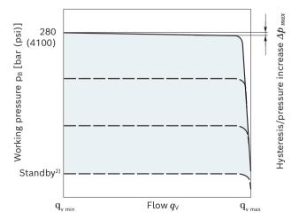
Characteristic curve valid at  $n_1$  = 1500 rpm and  $\theta_{fluid}$  = 50 °C (120 °F).
