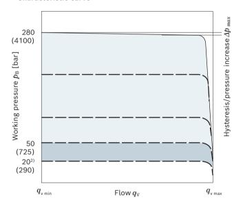
Characteristic curve valid at  $n_1$  = 1500 rpm and  $\theta_{fluid}$  = 50 °C (120 °F).
