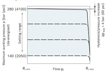
Characteristic curves valid at  $n_1$  = 1500 rpm and  $\vartheta_{fluid}$  = 50 °C (120 °F).
