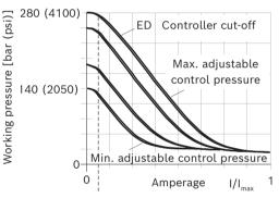
Setting point (control current for start of control at  $p_{max}$ )
