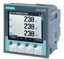
SENTRON, measuring device, 7KM PAC3200, LCD, L-L: 690 V, L-N: 400 V, 5 A, 3-phase, Modbus TCP, optional Modbus RTU / PROFINET / PROFIBUS, apparent/ active/reactive energy, class 0.5 acc. to IEC61557-12 or class 0.5s acc. to IEC62053-22, wide-range pwr sup. unit AC/DC, screw terminals
