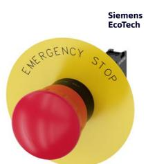
EMERGENCY STOP mushroom pushbutton, 22 mm, round, plastic, red, 40 mm, positive latching, acc. to EN ISO 13850, rotate-to-unlatch, with yellow backing plate, inscription: EMERGENCY STOP, with holder, 1 NC, screw terminal
