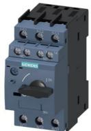
Circuit breaker 32 A A-release 27...32 A, N-release 400 A, for motor protection, class 10, screw connection, standard switching capacity, w. transverse AUX. switch 1 NO + 1 NC
