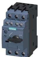
Circuit breaker 16 A A-release 11...16 A, N-release 208 A, for motor protection, class 10, screw connection, standard switching capacity w. transverse AUX. switch 1 NO + 1 NC
