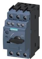
Circuit breaker 4 A A-release 2.8...4 A, N-release 52 A, for motor protection, class 10, screw connection, standard switching capacity, w. transverse AUX. switch 1 NO + 1 NC
