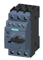
Circuit breaker 2.5 A A-release 1.8...2.5 A, N-release 33 A, for motor protection, class 10, screw connection, standard switching capacity, w. transverse AUX. switch 1 NO + 1 NC
