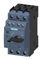
Circuit breaker 1 A A-release 0.7...1 A, N-release 13 A, for motor protection, class 10, screw connection, standard switching capacity, w. transverse AUX. switch 1 NO + 1 NC
