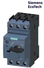
Circuit breaker size S00 for motor protection, CLASS 10 A-release 3.5...5 A N release 65 A screw terminal Standard switching capacity
