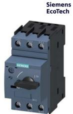
Circuit breaker size S00 for motor protection, CLASS 10 A-release 0.9...1.25 A N-release 16 A screw terminal Standard switching capacity
