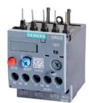
Overload relay 1.8...2.5 A size S00, class 10, for motor protection for mounting onto contactors main circuit: screw terminal AUX. circuit: screw terminal manual automatic reset
