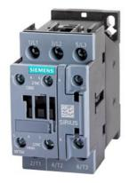
Contactor AC 220 V 50/60 HZ AC3 15 kW 400 V AUX contacts 1 NO +1 NC 3-pole, size S0 screw terminal
