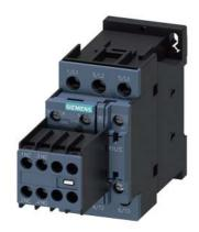
power contactor, AC-3e/AC-3, 12 A, 5.5 kW / 400 V, 3-pole, 230 V AC, 50 Hz, auxiliary contacts: 2 NO + 2 NC, screw terminal, size: S0, removable auxiliary switch
