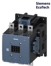
power contactor, AC-3e/AC-3 500 A, 250 kW / 400 V AC (50-60 Hz) / DC Uc: 220-240 V 3-pole, auxiliary contacts 2 NO + 2 NC drive: conventional main circuit: busbar control and auxiliary circuit: screw terminal
