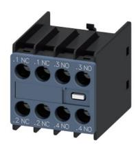
auxiliary switch, on the front, 2 NO + 2 NC, .1/.2, .1/.2, .3/.4, .3/.4, current path: 1 NC, 1 NC, 1 NO, 1 NO, screw terminal, for contactors 3RT2 and contactor relays 3RH2
