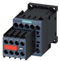
contactor relay, 6 NO + 2 NC, 230 V AC, 50 / 60 Hz, size S00, screw terminal, captive auxiliary switch
