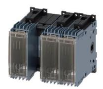
Switch disconnector with fuse 63 A, Size 1, 3-pole for LV HRC fuse Sz. 000 Front operating mechanism center Basic unit without handle Box terminal
