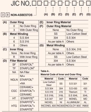
EX) JIC-3834-R-SF-304-SS means Graphite with 304 winding and inner & outer ring type. =Winding(Hoop) SS304, Filler: STARFOIL®, Inner Ring: SS304, Outer Low carbon steel
