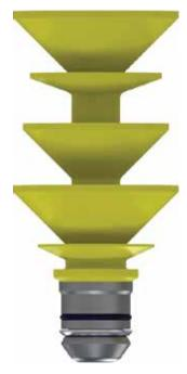
Weatherford's inner-string latch-in stinger dart is pumped behind cement and wipes the inside of drillpipe or tubing strings, providing a mechanical barrier between cement and spacer fluids or between mud and cement.
