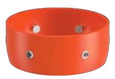
SledgeHammer's Slip on Set Screw Stop Collar is single piece collar that uses one row of set screws to induce the gripping force. It is used where high axial loads are expected, and is effective where low annular clearance is encountered.
