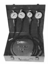
Trouble finding in the brake booster and capacity test after replacement of parts can easily be performed under the operational condition without removing them from the vehicle.
