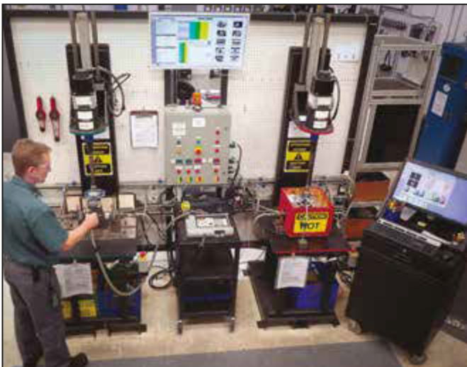
Velan's API 624 research and development test lab. Velan's R&D department is fully equipped for testing API 624, API 622, ISO 15848-1, and ISO 15848-2 as well.
